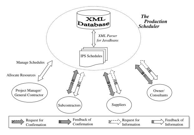
Figure 6: Structure of the IPS system model
