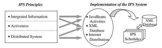
Figure 4: Proposed implementation of IPS principles with JavaBeans and XML
