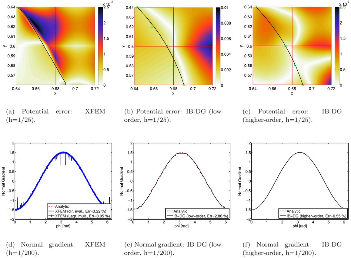
FIGURE 19. Dielectric-interface example: (top) detailed potential error  $|\Phi^h - \Phi|$ ,  $\Gamma$ -boundary and background mesh with control-points; (bottom) normal gradient along  $\Gamma$ -boundary.
