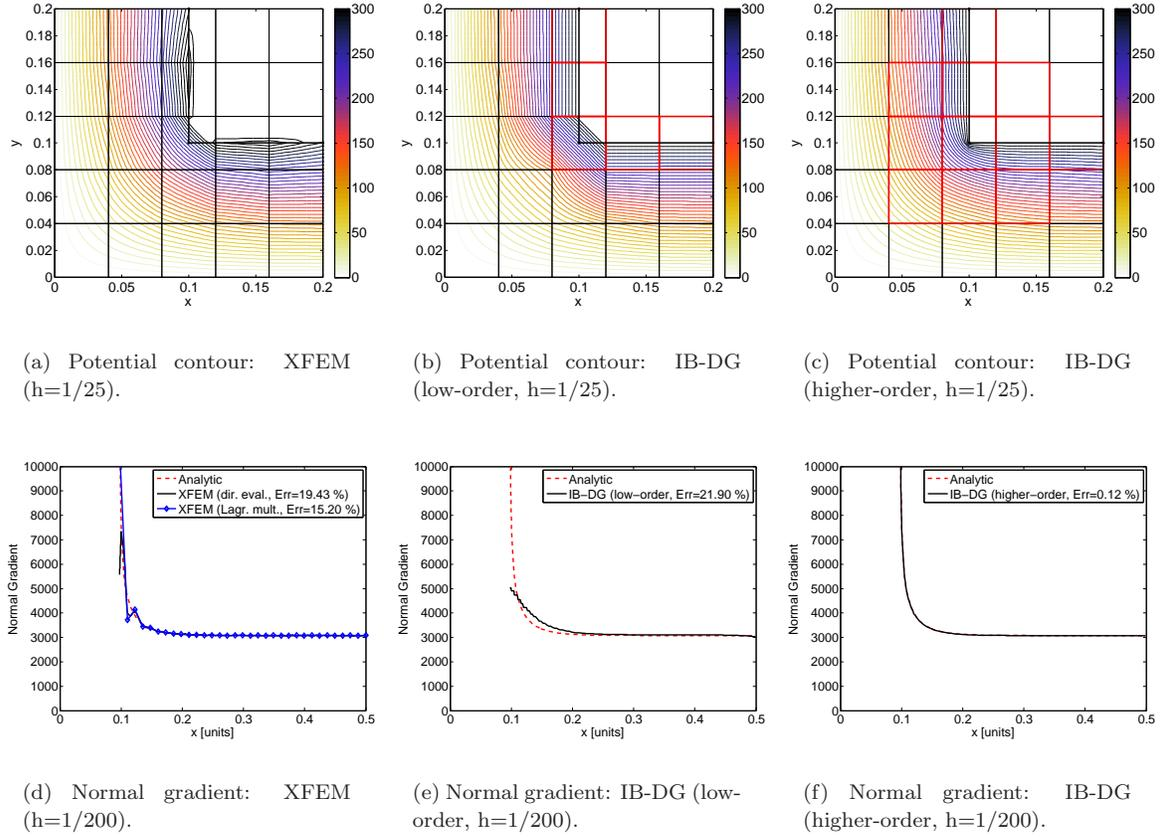
FIGURE 15. Corner example: (top) resulting potential contour,  $\Gamma$ -boundary and background mesh; (bottom) normal gradient along  $\Gamma$ -boundary.
