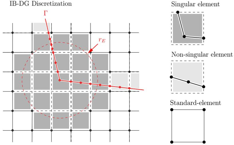
FIGURE 9. Singular element enhancement within enrichment radius  $r_E$ .
