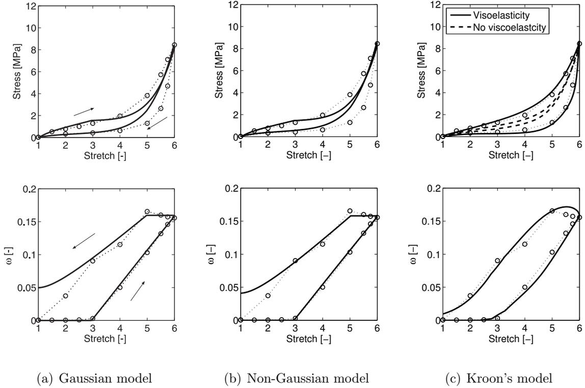
**Figure 2** Comparison of the sulfur vulcanized NR data (dotted line) to: (a) the Gaussian model; (b) the non-Gaussian model; and (c) Kroon’s model with (solid line) and without (dashed line) viscoelasticity. The curve for the degree of crystallinity is only plotted once because it stays the same for both cases. Optimized parameters for (a) and (b) can be found in Table 3 under NR-S.
