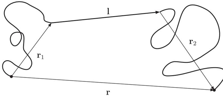
**Figure 1** Schematic of a partially crystallized chain between two crosslinks with end-to-end vectors of the two amorphous subchains  $\mathbf{r}_1$ ,  $\mathbf{r}_2$ , the crystal vector  $\mathbf{l}$ , and the chain end-to-end vector  $\mathbf{r}$ .
