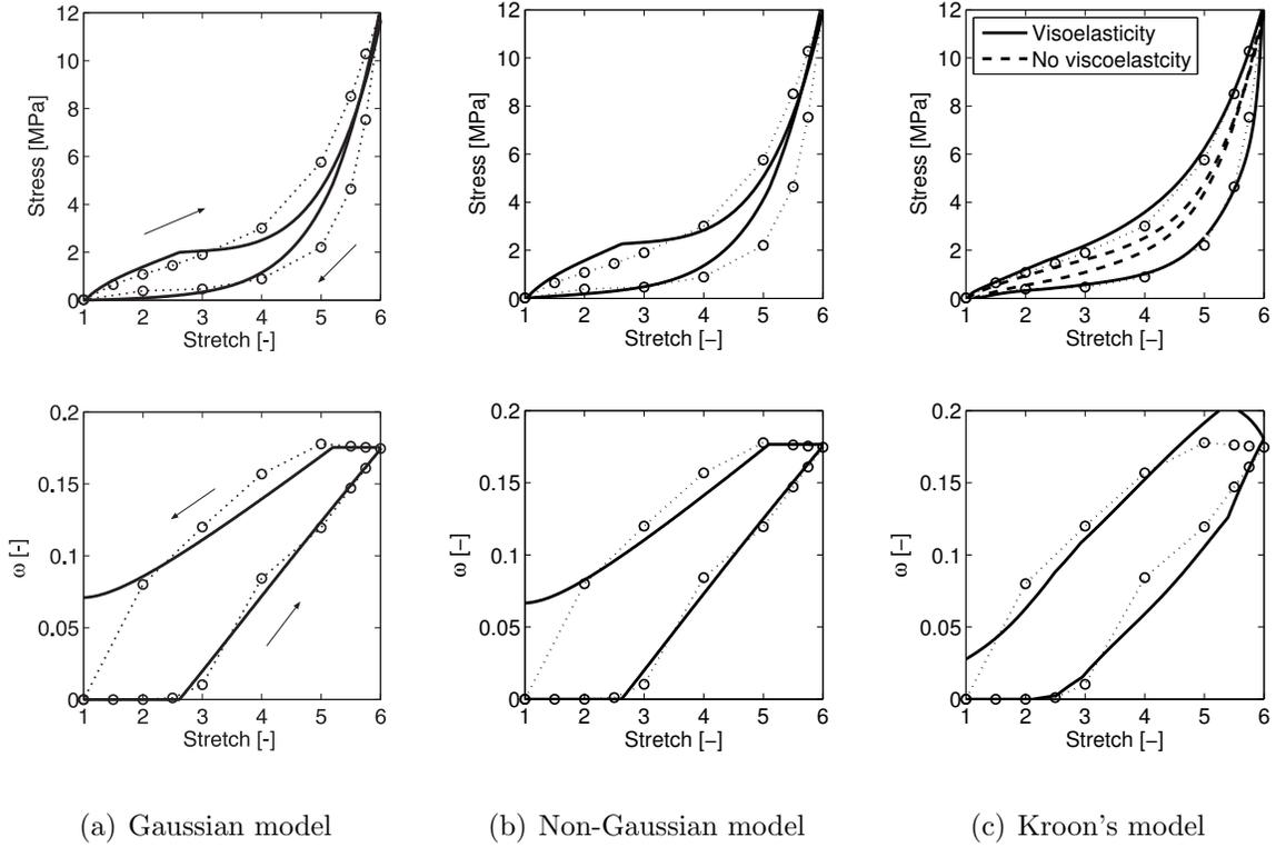
**Figure 3** Comparison of the peroxide vulcanized NR data (dotted line) to: (a) the Gaussian model; (b) the non-Gaussian model; and (c) Kroon's model with (solid line) and without (dashed line) viscoelasticity. The curve for the degree of crystallinity is only plotted once because it stays the same for both cases. Optimized parameters for (a) and (b) can be found in Table 3 under NR-P .
