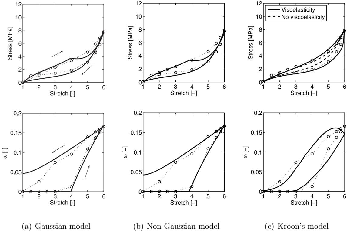
**Figure 4** Comparison of the sulfur vulcanized synthetic polyisoprene rubber data (dotted line) to: (a) the Gaussian model; (b) the non-Gaussian model; and (c) Kroon's model with (solid line) and without (dashed line) viscoelasticity. The curve for the degree of crystallinity is only plotted once because it stays the same for both cases. Optimized parameters for (a) and (b) can be found in Table 3 under IR-S.
