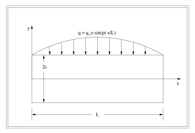
• The exact solution of the y-displacement along the centerline of a beam with the boundary conditions
