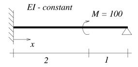
4. Find the equation for the deflection of the beam shown. Assume a constant value for EI. Use the given coordinate system.
