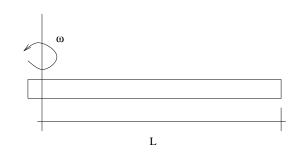
3. For the bar shown determine the displacement field u(x).
