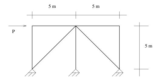
4. For the truss shown, determine its degree of indeterminacy.
