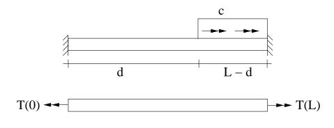
3. In the statically indeterminate beam shown, find the reactions at the wall by integrating the differential equation for the deflection of the beam.
