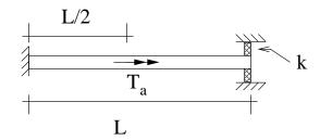
2. An elastic solid circular bar of length L with polar moment of inertia J and shear modulus G is built-in at both ends and subject to a system of distributed torques:
