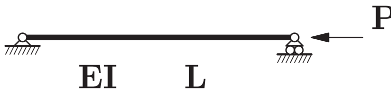
Figure 1: Simply supported beam
