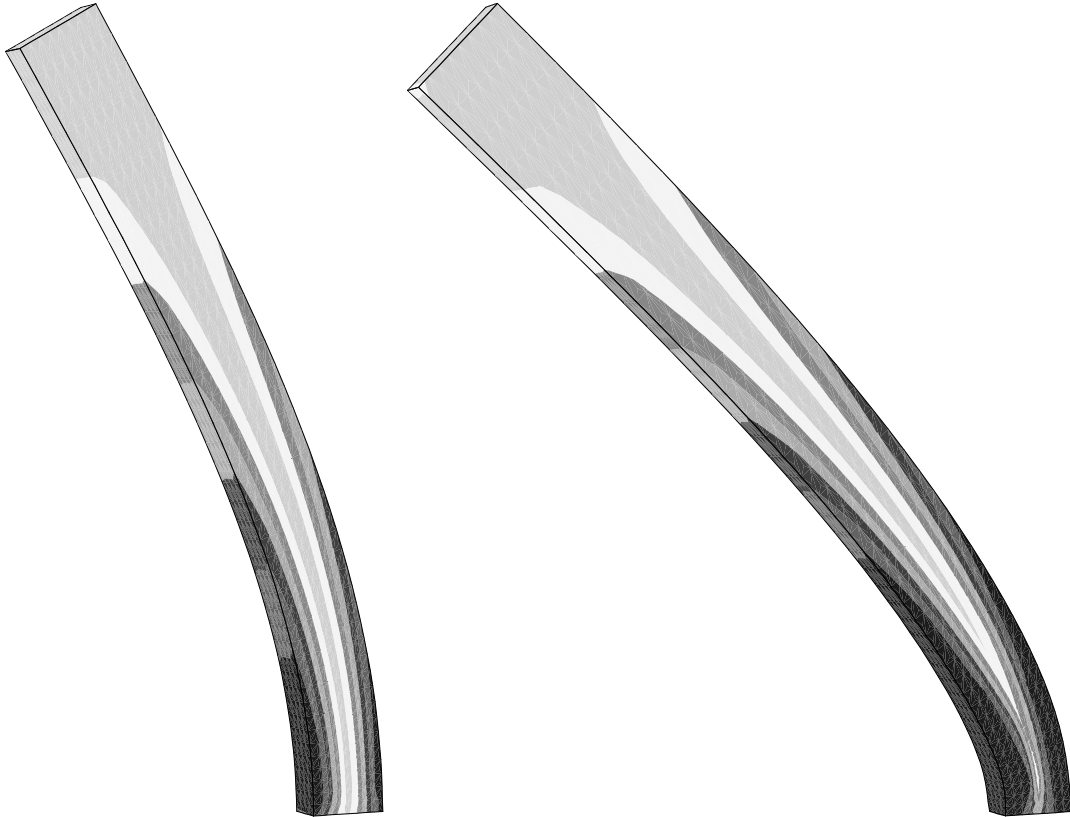
Figure 7: Cantilever Beam: Deformed Mesh at Steps 4 and 8
