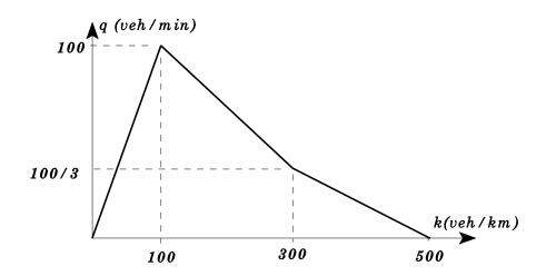
Construct a t-x diagram showing the vehicle trajectories and interfaces arising when a capacity stream of vehicles (q=100) is suddenly stopped (e.g. at t=0) at a railroad crossing. (Note that the q-k curve is not concave).
