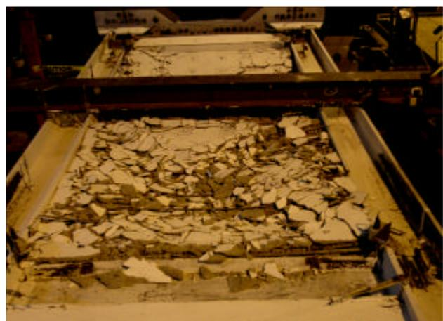
At the End of the Test at 7.3  $\delta$ y (Drift of 4.4%)
