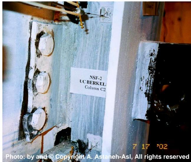
Figure 12. Onset of shear tab fracture thru bottom bolt hole edge distance; at W18x35 west of C2 after Test NSF 2.
