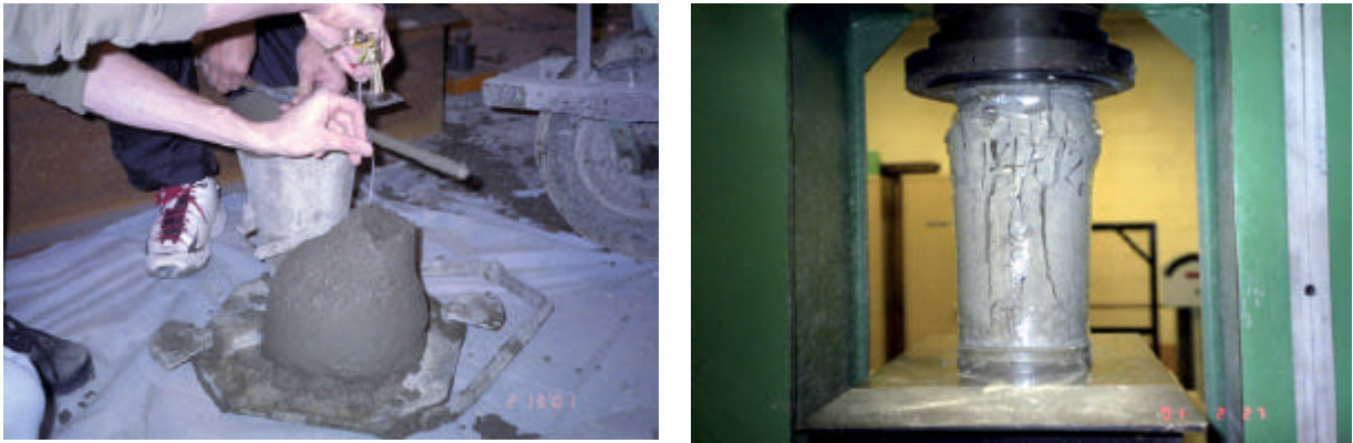
Figure 2.9. Slump Test and Cylinder Tests on Concrete Used in Slab
