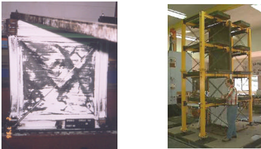
Figure 6. One-story and four-story specimens (Rezaei, Ventura and Prion, 2000) (Photos courtesy of Prof. C. Ventura.)
